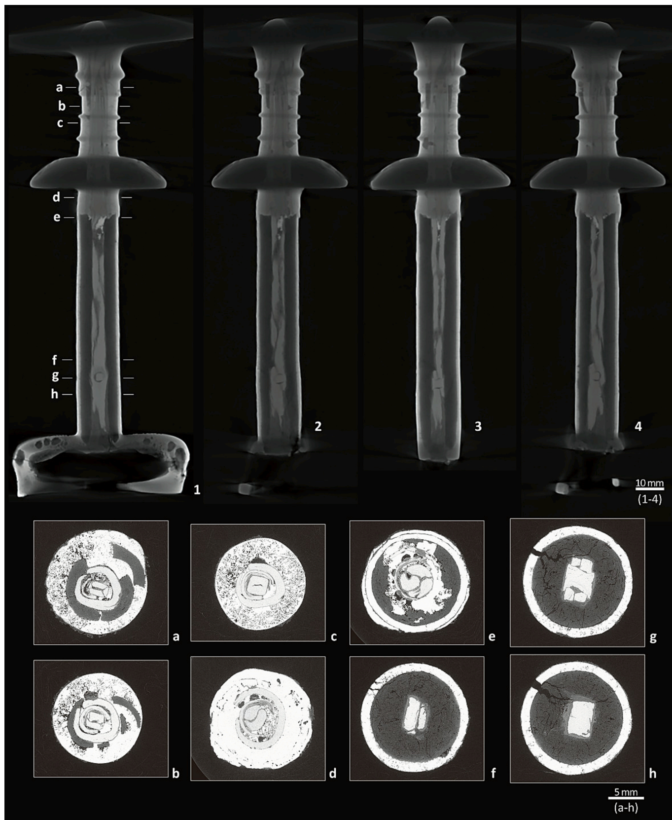
Fig. 7. No. 513: (1, 2, 3, 4) X-ray projection images of the hilt using inspeXio SMX-225CT FRD HR; (a-h) Tomographic sections of the hilt using SPring-8.
